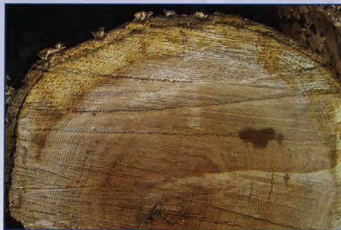
Figure 1. Sapwood decay organisms invade trees after the bark and cambium have died. The decay proceeds from outside the stem toward the center.
